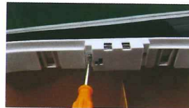
安装紧固螺丝2个 Screw in 2 screws
