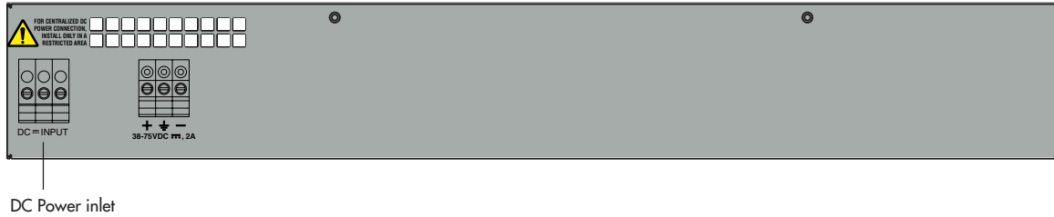
Figure 2: DC Power inlet terminals on an AT-8724XL.
