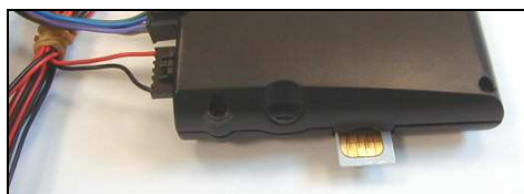
Figure 6 - SIM Card insertion
